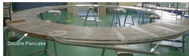
Fig. 4. Double pancake of EF4 coil after thermal curing.
