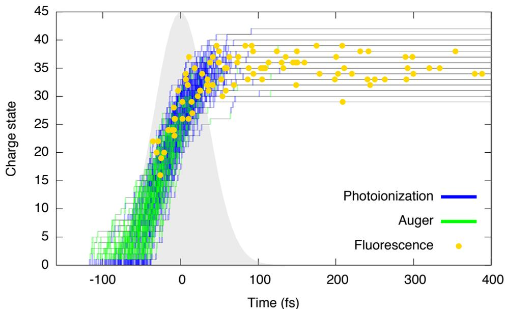
Figure: Exemplary pathways of multiphoton multiple ionization dynamics of Xe at 4.5 keV.
