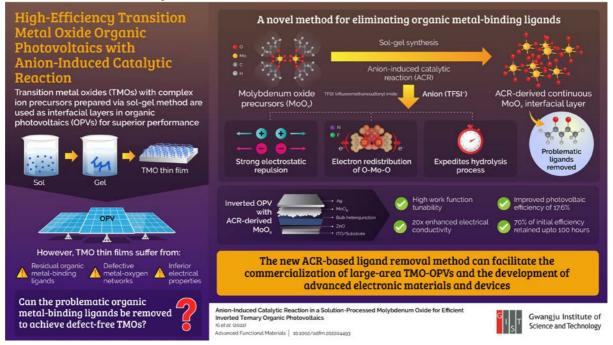
Image title: Removing residual organic metal-binding ligands with anion-induced catalytic reaction (ACR).
