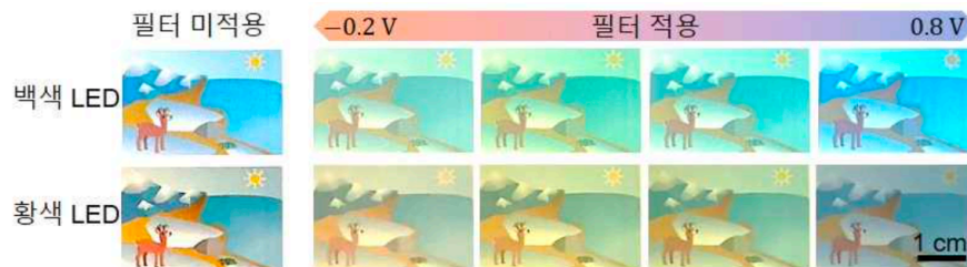
▲ Optical filter that maintains the color of an object even under differently colored lighting
