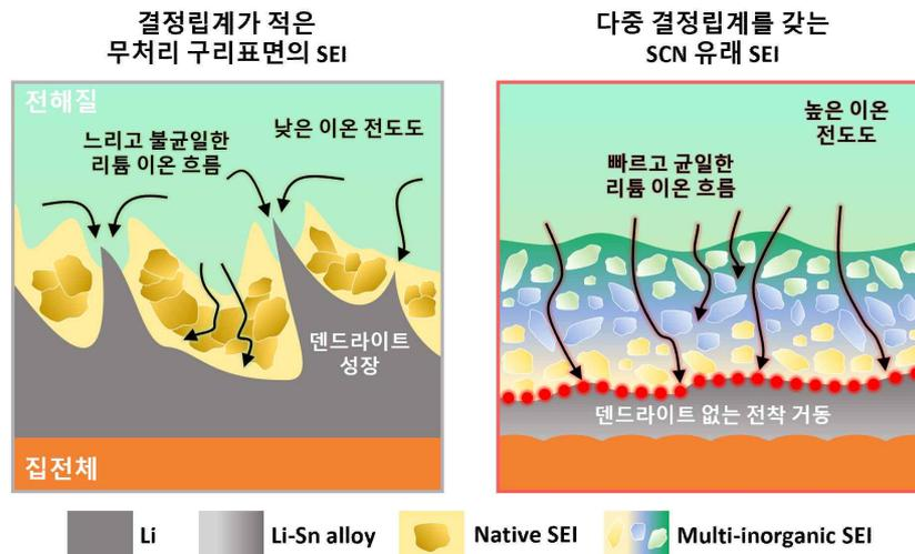
▲ Schematic comparison of a native solid electrolyte interface (SEI) formed on an untreated copper (Cu) surface with low grain boundary density and a solid electrolyte interface (SEI) derived from SCN with multiple grain boundaries. The SEI formed from the nanowire precursor (SCN) exhibits high ionic conductivity, leading to uniform lithium ion transport, effectively suppressing dendrite growth and achieving stable lithium deposition.
