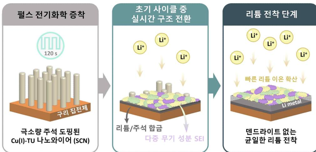
▲ *Schematic diagram of the lithium electrodeposition step. This depicts the process by which lithium/tin alloying and a multi-inorganic SEI are formed in real time during the initial cycle on an SCN current collector manufactured by pulsed electrochemical deposition, resulting in uniform lithium ion diffusion and dendrite-free lithium deposition.*
