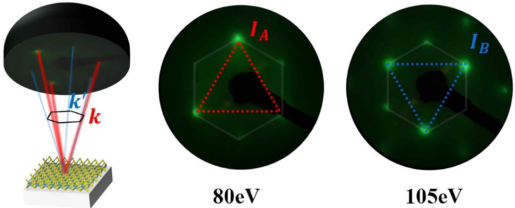
▲ *Non-destructive single crystal quality verification: By varying the electron beam energy and measuring the change in brightness of the diffraction pattern spots, the team can determine whether and to what extent "twin crystals" with flipped atomic arrangements are present.*
