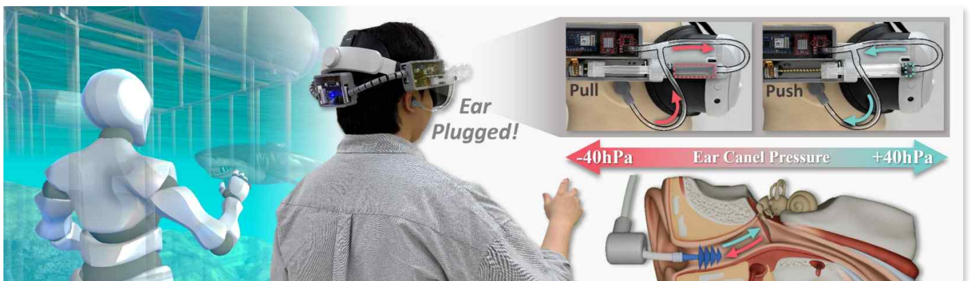
▲ Overview of the EarPressure VR System. This wearable haptic feedback device measures and analyzes changes in atmospheric and water pressure in a VR environment in real time, precisely controlling the pressure in the ear canal within a range of \pm 40 hPa. This allows users to experience the sensation of ear-popping, similar to the sensation experienced when descending underwater or ascending to high altitudes.
