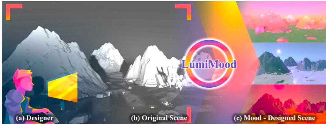
▲ LumiMood system overview. LumiMood receives a 3D background as input from the designer and creates the atmosphere of the scene by adjusting lighting and post-processing effects.
