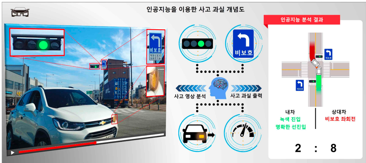
[Figure 3] Conceptual diagram of traffic accident error evaluation technology using artificial intelligence
