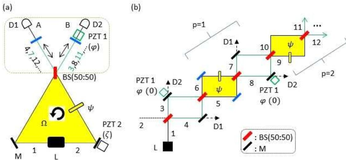
▲ (a) Quantum ring laser gyroscope structure. (b) Infinite series of CBW as a group of friends
