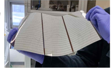
▲ Schematic diagram of the structure of a large-area flexible organic solar cell module (left) and actual photo (right)
