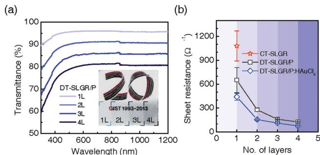
**Figure 5.** a) Optical transmittance spectra of one- to four-layer DT-SLGR/P films. The inset shows a photograph of an offset-stack of four DT-SLGR/P layers on a fused silica substrate. In the inset, the number of layers in each area is marked. b) Variations in the  $R_S$  of the CT-SLGR (star), DT-SLGR/P (squares), and  $\text{HAuCl}_4$ -doped DT-SLGR/P (diamonds) films as a function of the number of layers.
