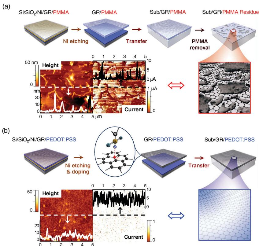
**Figure 1.** Schematic illustrations and representative *c*-AFM data for the a) CT and b) DT methods. PMMA (80 nm) and PEDOT:PSS (50 nm) were used as the supporting film in the CT and DT methods, respectively. Representative *c*-AFM height images (left) and current images (right) for both the CT-GR (a) and DT-GR/P (b) films are shown. The inset graphs show the height and current profiles along the dashed lines. The inserted illustration in (b) shows a doping mechanism of GR by PEDOT:PSS.
