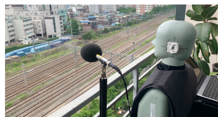
Environmental noise recording using a 2-channel noise measurement system
