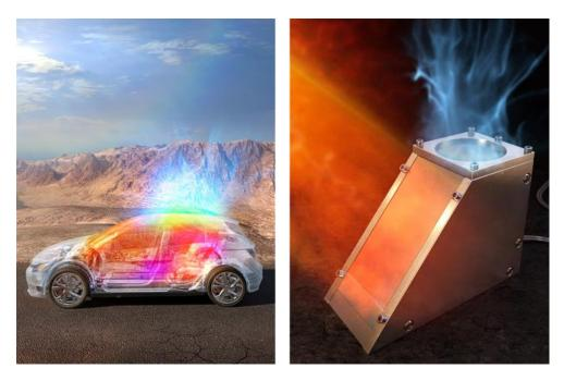
The bottom layer of the Janus emitter absorbs the heat inside the vehicle and emits it through the top layer to the atmosphere (indicated in blue), causing a temperature drop. The right image shows an experimental model that simulates a vehicle.
