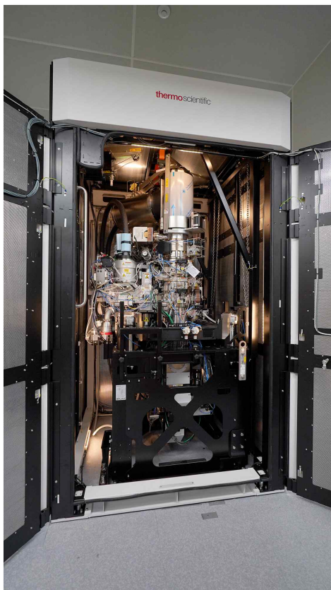
▲ The 10th state-of-the-art 300kV (kilovolt) high-resolution cryogenic transmission electron microscope (300kV Cryo-EM) installed in the Advanced Institute of Instrumental Analysis (GAIA)
