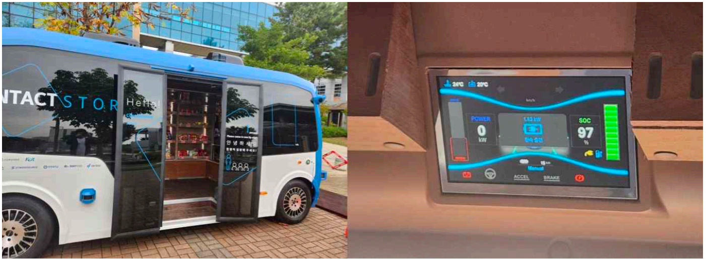
▲ Photo of a non-face-to-face smart store service vehicle (left) and a power monitoring device installed inside the vehicle (right)
