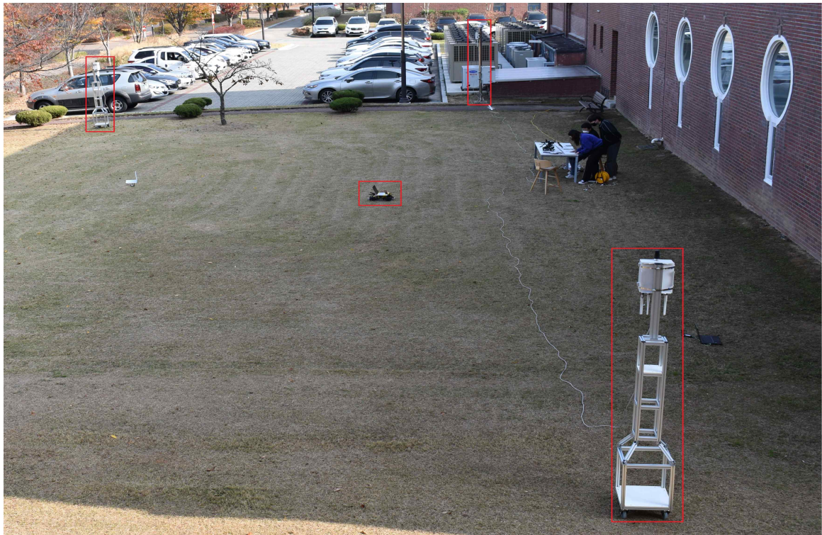
▲ Hybrid-V2X ToF-based positioning verification scene using RSU (3 locations) and OBU (Motor Vehicle)
