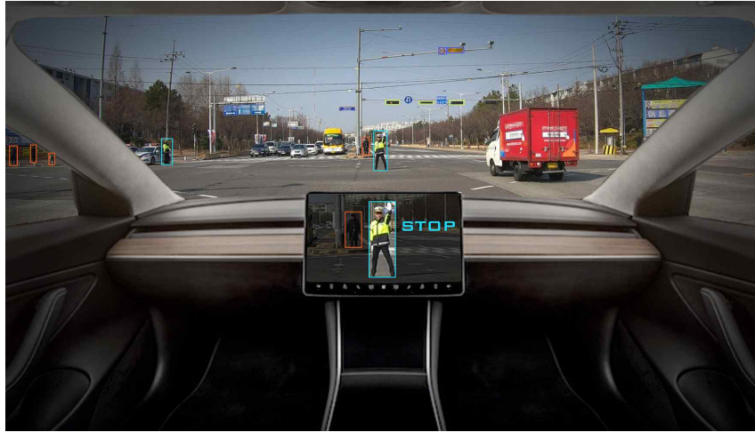
[Figure 2] Recognizing a policeman and hand signals in a self-driving vehicle (Korean Image)
