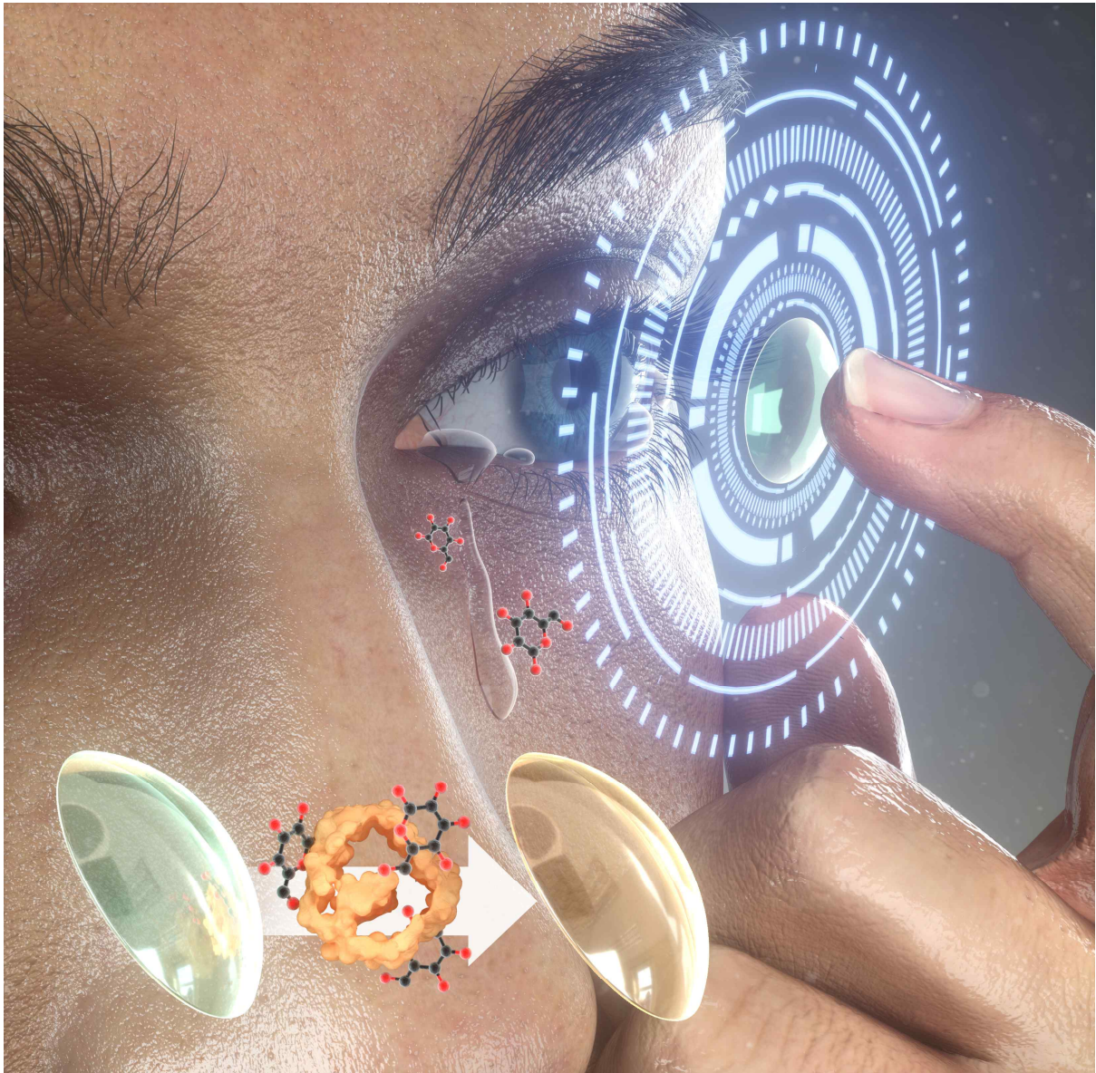
▲ Schematic diagram of color change to smart contact lenses due to glucose in tears
